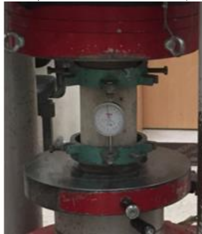
Figure 4. Mortar compression test and strain measurement. (Self-Elaboration).
