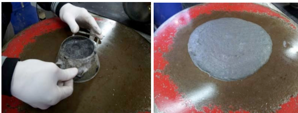
Figure 2. Slump test for assessing consistency of UHPC
