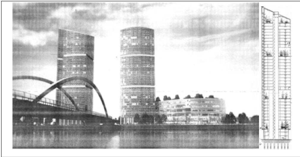
Figure 11. The greening of the roof of block "A" and the arrangement of winter gardens in the high-rise blocks "B", "C" and "G" of the multifunctional complex on Rybalsky Island, Kiev
