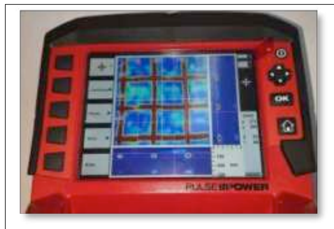
Figure 6. FerroScan PS1000 Equipment - Reinforcement Information
