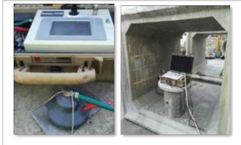
Figure 14. PermeaTorr Equipment - Air Permeability
