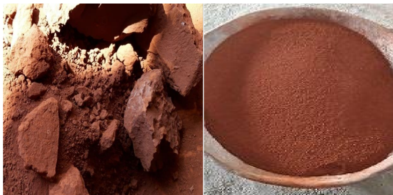
Figure 2. Raw iron ore tailings and crushed iron ore tailings
