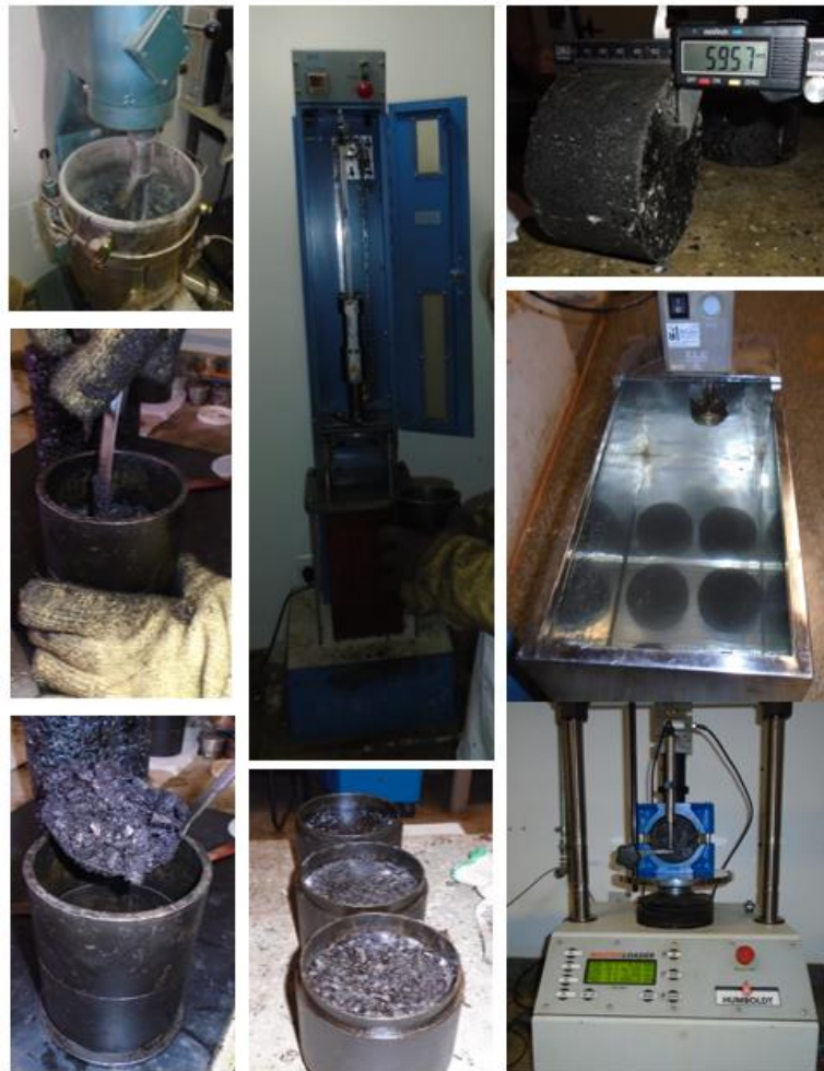
Figure 3. Dosage procedure by Marshall Method at laboratory
